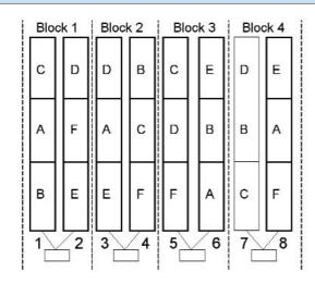
Six different mixtures of feedstock wastes were composted using EcoPOD® in-vessel composters Each of the 8 EcoPOD®s was divided into 3 sections to allow replication of each mixture (x 4) in a randomised complete block experiment.
