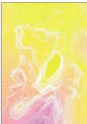
Fig. 4 Contour data were coded for elevation to produce this digital elevation model (DEM). The pink colours represent the highest ground in the vicinity of Penrhyn Quarry.
