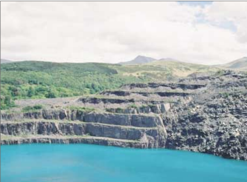
Photo 3. Galleries preserved at Penrhyn Quarry; they served to facilitate the extraction of usable slate and also the rapid removal of rubbish from the working face, often by tram.
